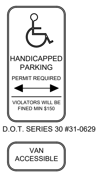
HANDICAPPED PARKING SIGN DETAIL N.T.S.
